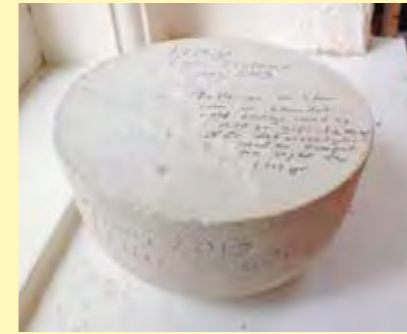
Plaster object, which occupies a volume of exactly 1 litre, cast in a rubber bowl with 1000 g of plaster and 600 g of water, as part of an experiment to determine the correct proportions of water and plaster to be used in the process.
