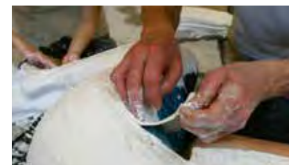
You make the first half of the shell and build up a thick edge. This edge is lubricated before you build the next shell up against it.
