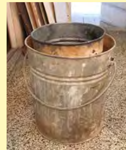
Normally, the glue was melted in a 15 liter galvanized tin bucket, which stood on a brick in a 30 liter tin bucket of water, which stood on a gas stove to keep the water boiling.
