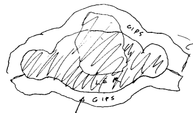
Seen from above. In the one half-part of the mould, the shape ought to facilitate the eventual removal of the mould-piece.
