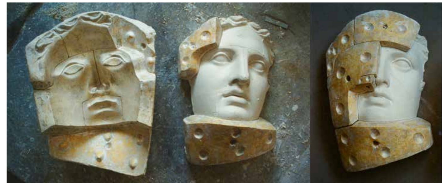
Generally, the eye of a steel-thread is cast into the wedge-pieces, offering the special advantage that later on, during the casting process, through a hole in the main piece, these wedge-pieces can be fastened together with twine.
