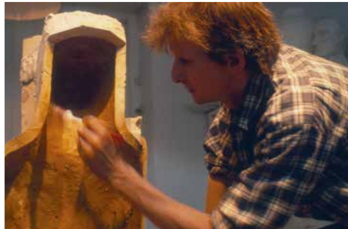
The mould is smeared with stearin/rapeseed oil.
