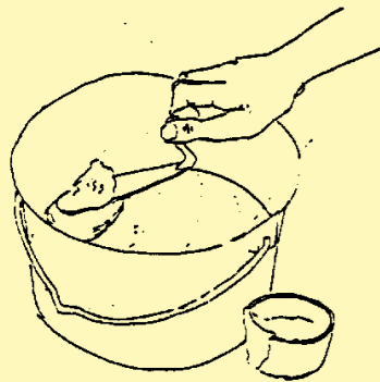
Use the plaster from the one side of the bucket to the other.
