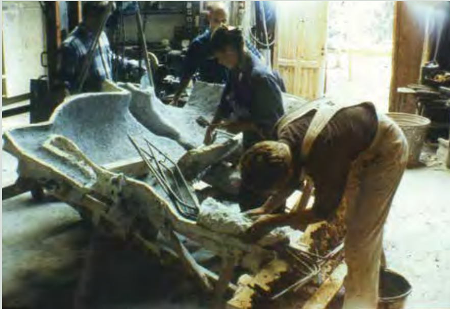
Equestrian statue in concrete by Ole Barslund (1968-) — The equestrian statue was cast in fibre-concrete in a waste-plaster mould by Ole Barslund in 1994, at the time that he was a student at The Sculpture School. It was cast in fibre-concrete in a waste-plaster mould. The body of the horse was cast as a shell in fibre-concrete, and weighed about 500 kg. The three bearing legs, each of which measures about 10-15 cm at the thinnest points of the legs, were reinforced with ten carefully placed 10 mm ribbed round stainless steel bars. The socle was almost solid and weighed approximately 500 kg.
