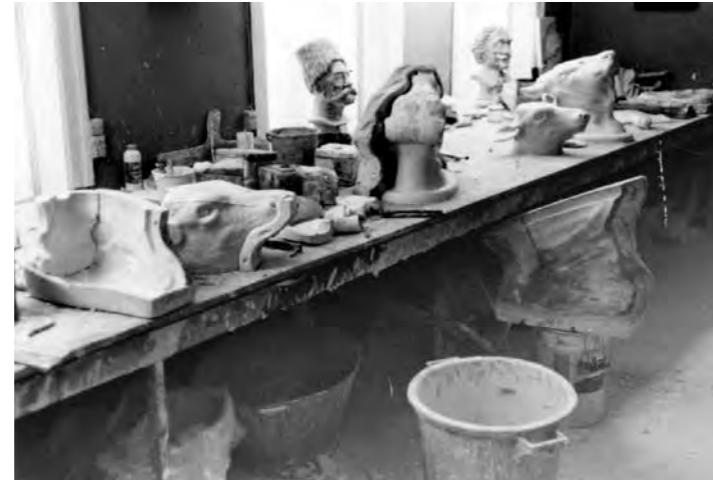
Photo from the stucco workshop Agnbak stuk at Lindgreens Allé 6. Casting of plaster cows' heads, for butcher shops.
